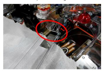
4. Loosen the two cross screws of the posts (where the ramp was pulled out).
