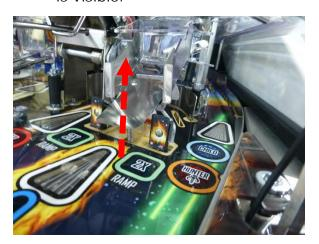
2d) Place the 2 mm thick Ramp Washer in the indentation of the playfield (flush with the oblong hole). Remove the foils from the plastic beforehand!
