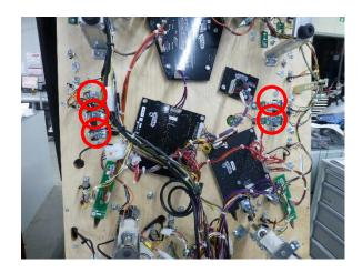
1b) Loosen the two screws of the targets with a ¼" socket wrench.
