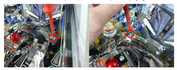
2c) Lift the ramp at the front by the metal tab so that the threaded metal pin is visible.
