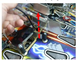
6d) Clamp the plastic angle between the two screw heads of the ¼" screws. Remove the foil from the plastic angle beforehand.
