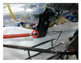
4b) Put the supplied metal bracket on the screw and fix it with the nut.
