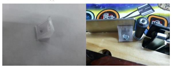
5e) Reinstall the original plastic and secure it with the two Phillips screws and the 5/16" nut.
