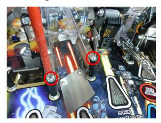
6c) Lift the ramp at the front by the metal tab so that there is space between the ramp and the playing field.
