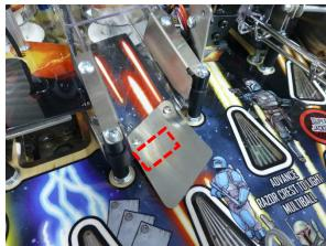
6f) Reattach the ramp to the playing field. Place the two black spacers between the metal angle and the post and fasten them with the Phillips screws. Note: Right long spacer with long screw, left short spacer with short screw.
