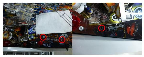
5b) Carefully remove the plastic upwards and turn it slightly to the side. If possible, place a cloth under the plastic to avoid scratches.
