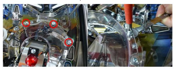
3b) Remove protective films from the Anti-Airball-Plastic and place it under the original plastic.
