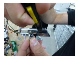
1e) Glue on new foam pad (small target pad).
